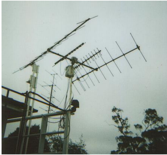
Above... Pairs of 2 metre and 70cm yagis and rotators for doing satellite comms.
