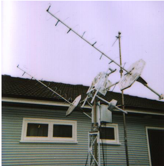
Above ... A pair of 70 cm band helicals and Alt/Az rotators also for space comms.
